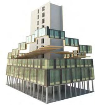
Modular system of interlocking prefabricated components with centralized concrete access core.
