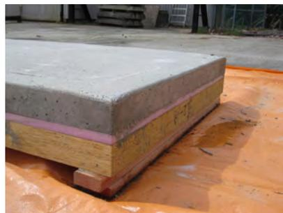
Composite floor panel used for testing
