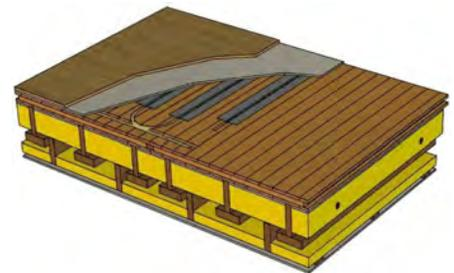
Horizontal panel showing hydronic heating channels.
