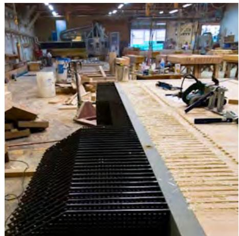
Installation of HSK perforated steel connectors.
