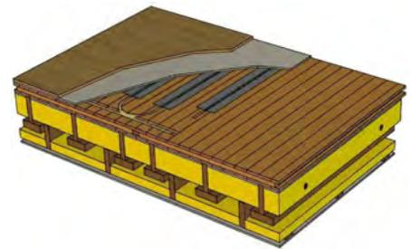
Horizontal panel showing hydronic heating channels.
