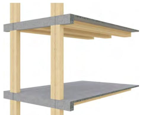
Hybrid floor slab and double wood columns comprise the load-bearing timber structure
