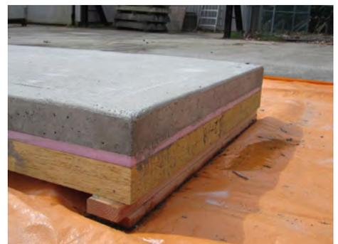
Composite floor panel used for testing.
