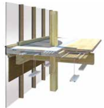
Detail of CLT floor panel system Rendering: MGA
